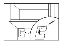
1 Attach brackets and prep hood for electrical connection
